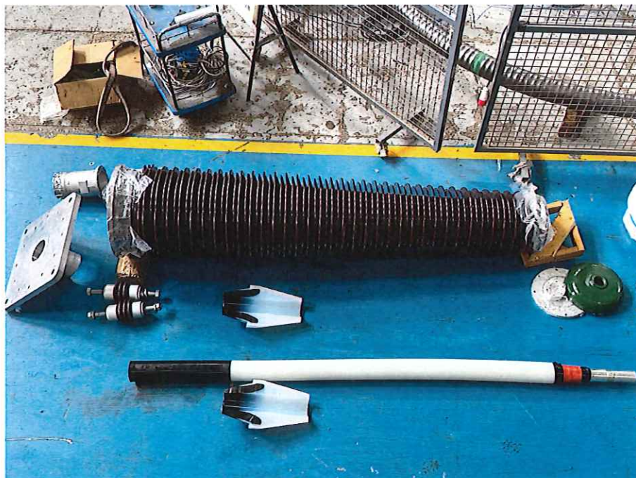
D2 瓷套式终端检查 Examination for porcelain type outdoor termination (2/2)
