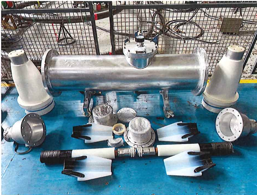
D11 GIS终端检查 Examination for GIS termination (3/3)
