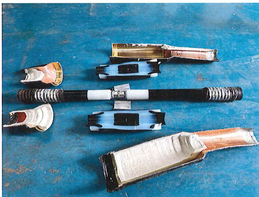
D8 直通接头检查 Examination for straight joint (2/2)
