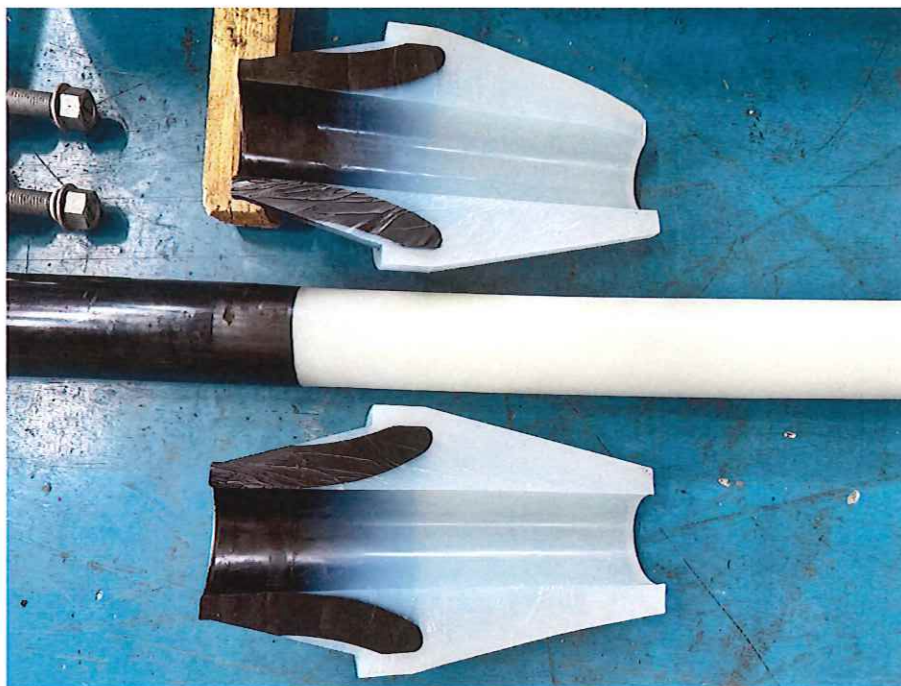
D3 复合套式终端检查 Examination for composite type outdoor termination (1/2)
